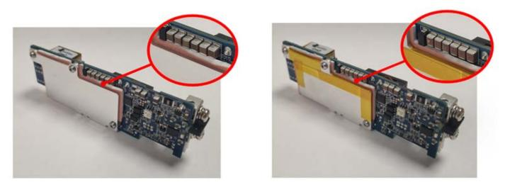
By adding a layer of tape to the edge of the heat sink, the required 2.5 mm Creepage and 2 mm Clearance for 1 MOPP is also met.
